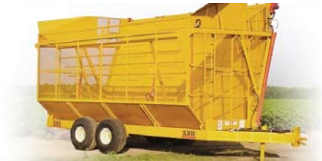
Figure 2 The boll buggy is used to transport harvested cotton between the harvester operating in the field and the module builder located at the edge of the field. (Photo courtesy of KBH, Inc.)
