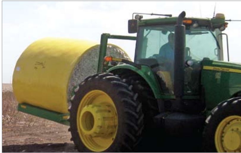
Figure 17 Carrying a round module with a three-point hitch attachment. The module is being staged for transport to the gin.
