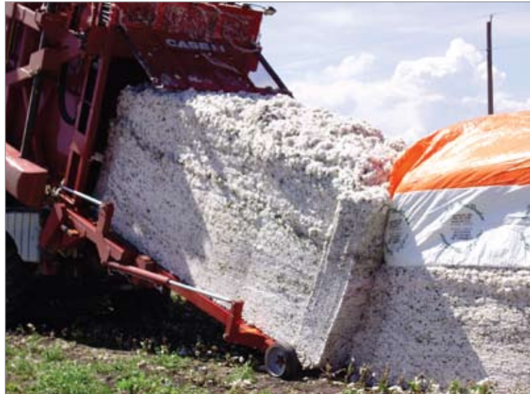
Figure 14 Half-length module unloaded too close to another module. Notice how the first module is pushed backward at the top. If this occurs before the module is covered, cotton will often fall off the back of the first module. Note also the offset between the two modules. This offset will make picking up the two modules together more difficult.
